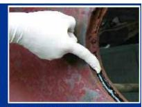
Press and contour bead into seam.
