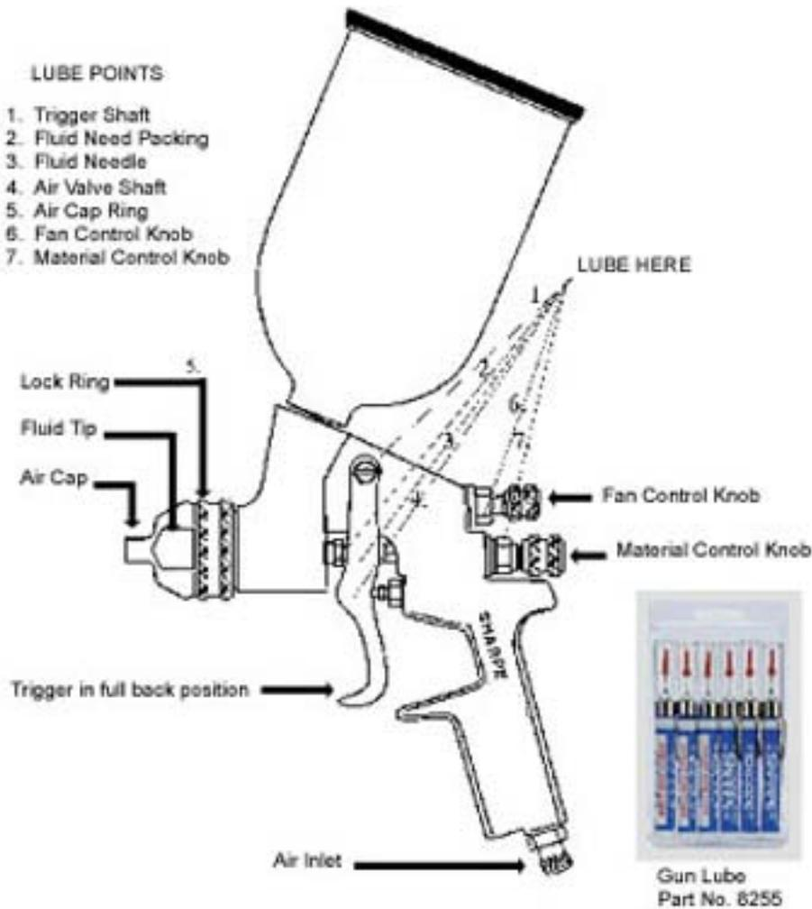
1. The spray gun should be lubricated after every cleaning using SHARPE gun lube. Place a drop on all moving parts, as shown in illustration.
