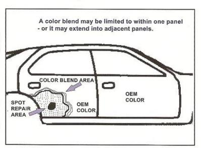
Because of the color variances or "color drift" in the typical OEM finish, obtaining a "butt" match (panel to panel) would be due almost exclusively to luck. PPG has excellent factory and intermix color matches but since we are trying to match such a broad range of OEM paint variables, blending is a necessity. Consider the following list of appearance factors that a technician faces when matching an OEM finish:
